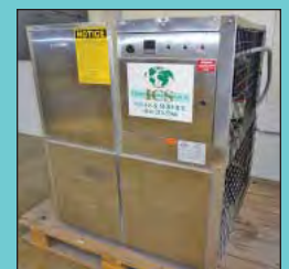
3 Ton ICS Model MSA-003-SCS Chiller
